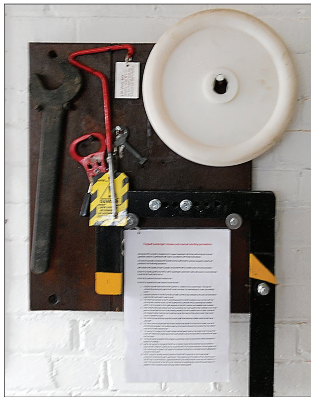
We also included a LOTO device and the bespoke door release key, as pictured above, with white label attached.
