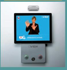
VIEW has made elevator emergency calls intelligent. Using sensors and artificial intelligence, emergencies, vandalism and unaccompanied objects are detected and reported autonomously to the emergency call center. This theoretically makes the emergency button superfluous because the guardian angel always goes with you.
