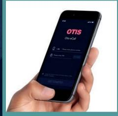
Otis eCall Plus is a smartphone app that provides a convenient and touchless passenger experience with two-button elevators. It allows passengers to place a destination call for an elevator from their phone to avoid any physical interaction with elevator fixtures. The app communicates with Bluetooth beacons installed near the hall buttons and inside the elevator near the car operating panel.
